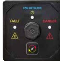
METHANE (CNG) GAS DETECTION 12/4 VDC 2-5/8 in. (76 mm) Square Current Draw @ 12 VDC: 40 mA One Integral Sensor
