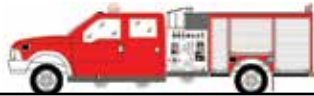
DARLEY VISION INITIAL ATTACK IA005 (CAFS Option Included) Pump (1000-1500) 300 Gallon Tank Copolymer Attack Body
