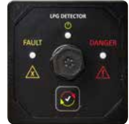
PROPANE (LPG) DETECTION 12/4 VDC 2-5/8 in. (76 mm) Square Current Draw @ 12 VDC: 40 mA One Integral Sensor
