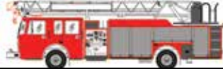
DARLEY VISION 78 AERIAL AR002 (CAFS Option Included) Pump (1000-1750) 500 Gallon Tank Copolymer Aerial Body
